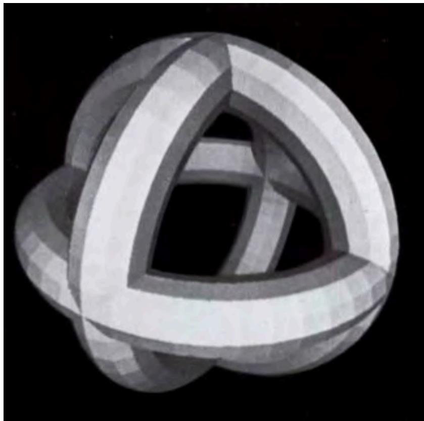
[Figure 8: Object shading using Warnock's hidden surface algorithm.]
