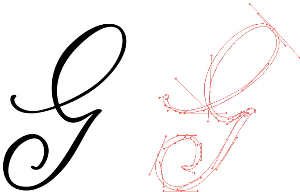
[Figure 6: Bézier curves used in digital typography design.]
